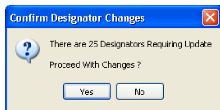
Figure 15. A prompt informs you how many designators will be updated when Tools » Force Annotate All Schematics is launched.
