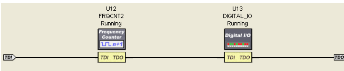
Figure 40. Virtual instruments are presented in the Soft Devices chain, once the FPGA is programmed.
