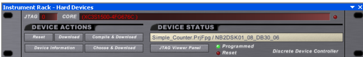
Figure 30. Instrument panel for the physical FPGA device.
