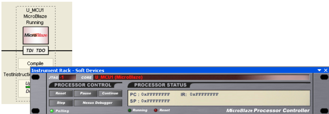
Figure 16. Accessing debug features from the processor's instrument panel
