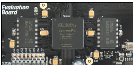
Figure 14. On-board SRAMS, U5 & U6
