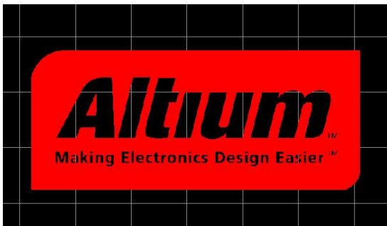
A logo converted into a series of PCB tracks by the example PCB Logo Creator script.
