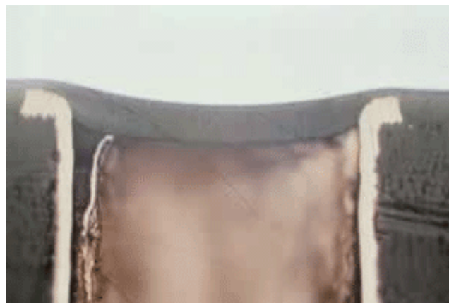
High current can melt Via plating
