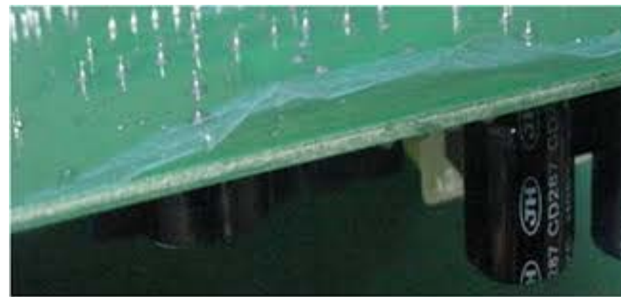
Heat can warp or delaminate the board
